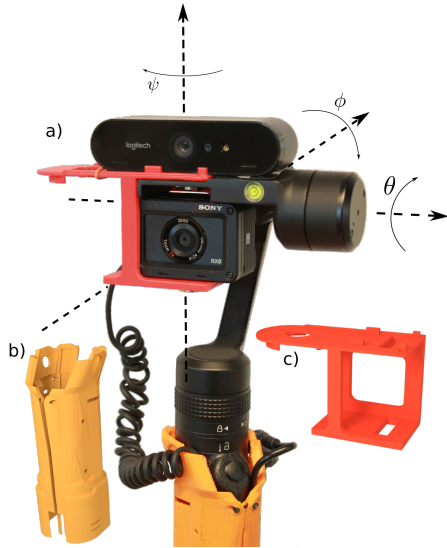
Fig. 3. a) Camera frame axes with pitch ( \theta ), roll ( \phi ), and yaw ( \psi ). The LookOut controller drives the orientation of the camera assembly. On top is the guide camera, while the bottom camera is the "star" camera. b) Gimbal handle enclosure to allow for wire pass through and a comfortable grip. c) Camera assembly engineered for balance, and alignment of camera optical axes.
