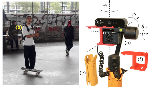
Fig. 2. A novice camera operator filming using the LookOut system: (a) An existing active camera gimbal, designed to stabilize mobile-phone filming. The mini-joystick is inactive by default. The orange 3D-printed handle channels the cables and protects the USB connectors from being bumped. (b) The backpack computer, connected to the gimbal by one USB cable and connected to (d) with another. Not shown, the backpack also has headphones and a lapel mic for two-way speech communication with the operator. (c) The primary “star” camera, recording high-quality footage to local memory. (d) The guide-camera, which has a wider field of view than (c), and whose video is fed to the backpack computer for real-time analysis. Star camera frame axes are represented with pitch ( \theta ), roll ( \phi ), and yaw ( \psi ). The LookOut controller drives the orientation of the camera assembly. (e) Gimbal handle enclosure to allow for wire pass-through and a comfortable grip. (f) Camera assembly engineered for balance and alignment of camera optical axes.
